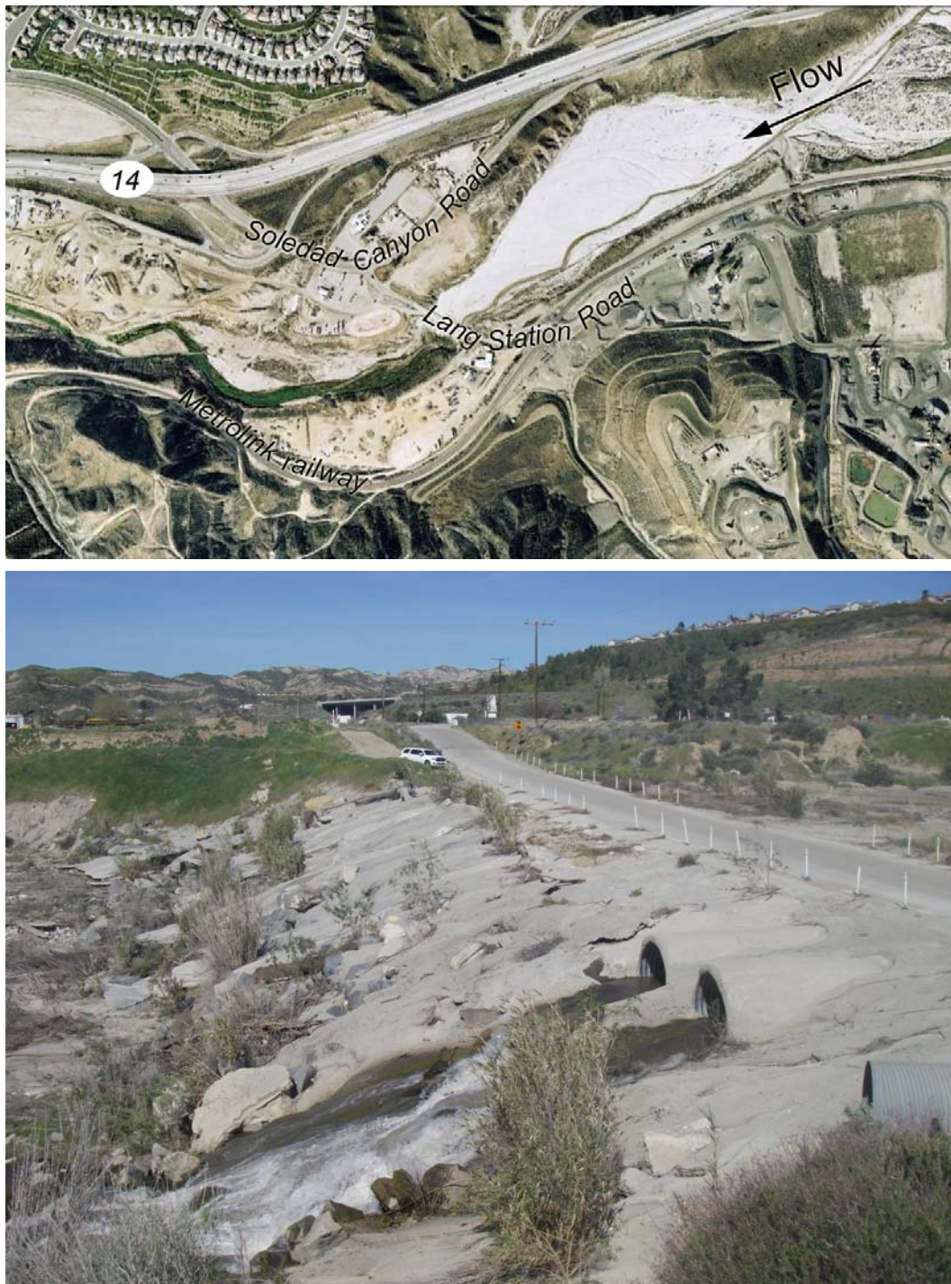
Figure 4-10. Lang Station Road and location of ongoing instream aggregate mining on the USCR near the mouth of Soledad Canyon. As visible in the NAIP 2006 aerial photograph (above), sediment is impounded on the upstream side of the 75 m (250 ft) long grade control structure. Active floodplain and instream aggregate mining is visible downstream. The bottom photo taken during our spring 2010 field surveys shows a profile view of the 5–6 m (15–20 ft) high crossing with the river's flow being routed through large culverts (flow direction is toward the left).
